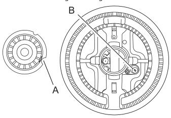
A electrode notch B ignition electrode Now fit the two trim rings, making sure that they are sitting down properly.
