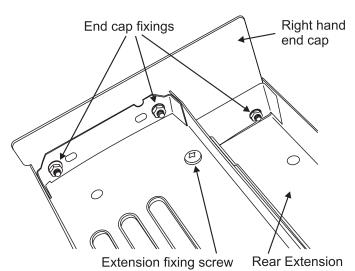
They are held in place by three fixing nuts on the inside face.
