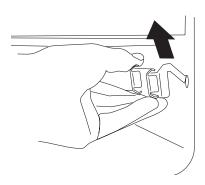
When you have finished, hook the side rails back onto the sides of the chamber. To refit the frame pull the side rails forward and for each side in turn support the side rail and press the frame down into the side rails. Replace the broiler pan.
