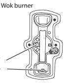
A orifice, B internal injector, C external injector Remove burner caps and heads. Remove old orifices, save the orifices removed from the appliance for future use. Fit new orifices. Reassemble in reverse order.
