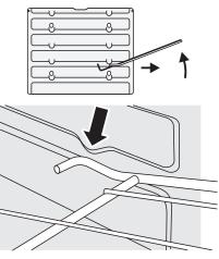
To refit the rack, line up the rack with a groove in the oven side and push the rack back until the ends hit the rack stop. Lift up the front so the rack ends clear the rack stops, and then lower the front so that the rack is level and push it fully back.
