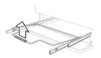
For safety, push the side rails back into the broiler chamber.
