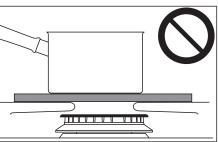
Simmering aids, such as asbestos or mesh mats, are NOT recommended. They will reduce burner performance and could damage the grates.
