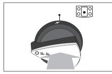
If, when you let go of the control knob, the burner goes out, the safety device has not held in. Turn the control to the off position and wait one minute, then try again this time holding in the control knob for slightly longer.
