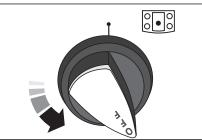
Adjust the flame height to suit by turning the knob. On this range the low position is beyond high, **not** between high and off. The 'LO' marks the low position. Turn the knob towards it after the contents of a pan have boiled.
