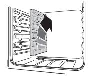
Once the linings are removed, the oven enamel interior can be cleaned.
