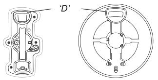
Turn the head until the 'D' matches the one on the burner base. Turn the head over and place it on the burner base.
