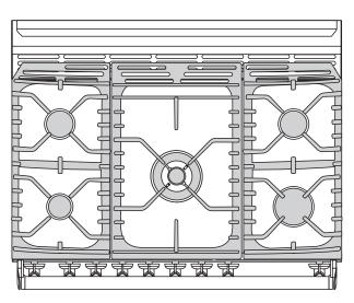
Each grate is different. Make sure that the grates are in the correct position and sitting down.
