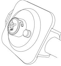
The regulator has a bayonet mounted top cap.
