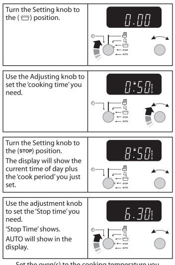
Set the oven(s) to the cooking temperature you need (don't forget to set a function if using the Multi-function oven).
