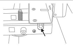
Make 10 complete (360°) turns clockwise. (This means turning and removing the leveling tool 20 times).
