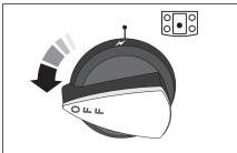
Keep holding the knob pressed in to let the gas through to the burner for few seconds. The igniter should spark and light the gas.
