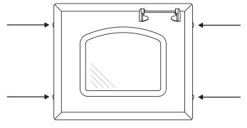
The fixing screws have a recessed hexagon socket in the head. A hexagon key to fit the screw is supplied in the instruction pack.
