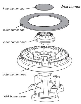
When reassembling a Wok burner, turn over the large base ring and find the 'D' shaped area.
