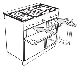
Open the broiler door and right hand oven door so that you can get a good grip on the bottom of the control panel as you move the oven.
