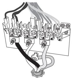
Fit the wires to the ground post and terminal block
