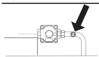
view from above with the flue grille removed Connect the appliance to the gas supply. Check the appliance is gas sound.
