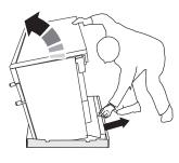
Repeat from the front and remove the front half of the polystyrene base.
