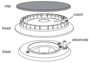
When refitting the burner head, make sure that the notch lines up with the electrode or hole in the base. Check that the burner head is level and that the cap is fitted centrally on the burner head.
