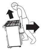
Do not move the range by pulling the door handles or knobs. Lift the front slightly and slide the range forward to disengage from the antitip bracket.
