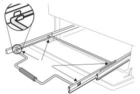
For each side, support the side rail with one hand and with the other hand life the frame up and out of the side clips.
