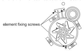
Remove the fixings that secure the element within the oven and lift the element away carefully. Disconnect the leads and connect to the replacement element and re-assemble parts in reverse order. Check that the oven operates correctly.
