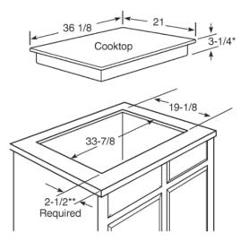
\*Depth of unit at conduit connection location (rear) is 6-1/4" on models PP975/945 and 4-3/16" on models CP350/650, PP944/962/932/912, and JP656/356/336. Depth of unit at baffle (front) is 4-5/8" on models PHP960/900.
