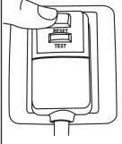
The power supply cord contains a current device that senses damage to the power cord. To test your power supply cord do the following:
