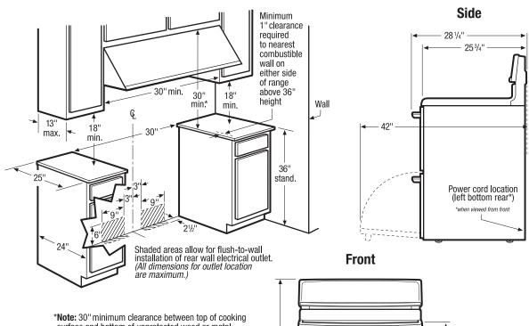
surface and bottom of unprotected wood or metal overhead cabinet; or 24" minimum clearance when bottom of wood or metal overhead cabinet is protected by not less than 1/4" flame-retardant millboard covered with not less than No. 28 MSG sheet steel, 0.015' stainless steel, 0.024" aluminum or 0.020" copper. 0" clearance is minimum for rear of range. Follow all dimension requirements provided above to prevent property damage, potential fire hazard, and incorrect countertop and cabinet cuts.
