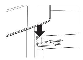
1 Lower the door onto the middle hinge pin.
