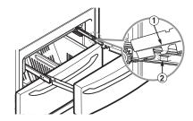
3 Lower the door into final position and tighten the screws located on both sides.
