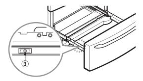
4 With the drawer pulled out to full extension, insert the basket in the rail assembly.
