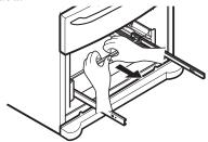
2 Grasp the drawer on each side and hook the door supports (1) into the rail tabs (2) located on both sides.
