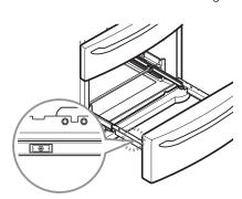
3 Grasp the drawer on each side and pull it up to separate it from the rails.
