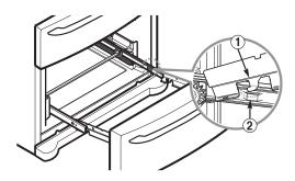
3 Lower the door into final position and tighten the screws located on both sides.
