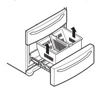
2 Remove the screws on both the left and right rails.
