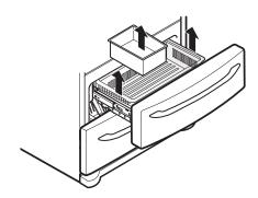
2 Remove the screws on both the left and right rails.
