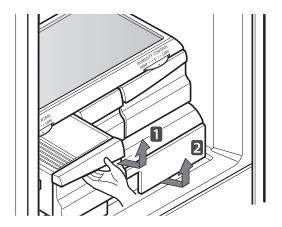
To install, slightly tilt up the front, insert the drawer into the frame and push it back into place.
