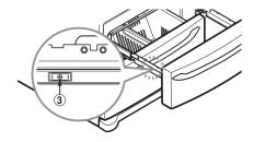
4 With the drawer pulled out to full extension, insert the basket and ice bin in the rail assembly.
