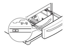
3 Grasp the drawer on each side and pull it up to separate it from the rails.
