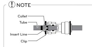
1) Gently press the Collet and insert the tube until only one line shows on the tube.
