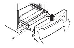
4 With both hands, flex the center bar enough to allow the gears on both ends to release from the track.
