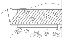
4. Excess water will flow through the drain outlet at the back of the machine and empty into the floor drain.
