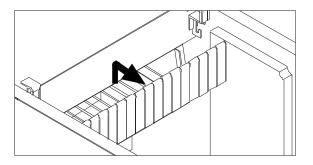
3. Remove the slideway from the water sump.
