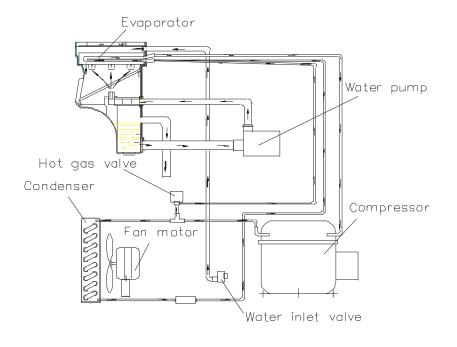
The ice maker begins with a fixed charge of water that is contained in the water sump. As the water is sprayed against the freezing evaporator surface, the portion of water that does not contain mineral impurities will freeze and stick to the ice cube molds. The water containing impurities falls back into the water sump. Gradually, during the
