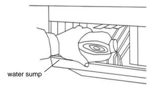
5. Allow 30 minutes for proper cleaning. After cleaning, shut off the power switch, and unscrew the nut of the water-draining hole on the rear of the unit. Drain off the water water to some container, and then screw the nut on tightly when the waste water is fully drained off.
