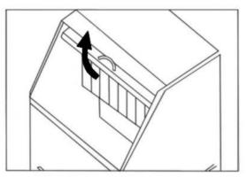
2. Take out the row of flake covers by snapping one end up and pulling forward.
