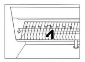
4. Find the sprinkler arm and raise it. Disconnect it from the water tube which is connected at the back of the sprinkler arm.
