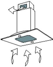
When installation of a ducted system is not possible or cost-effective, most Elica models can also operate as a Recirculating System, in which, dirty air is pulled through grease and charcoal filters, which remove grease, moisture, smoke and odors. The "purified" air is then recirculated back into the kitchen, instead of being vented outside.
