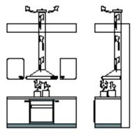
Most Elica kitchen ventilation products are designed as Ducted Systems, in which, dirty air from the stove top is pulled through a grease filter and then vented through a duct, directly into the outside air. This is the most powerful and effective ventilation method. Our one-way no-return valve, standard on all models, eliminates outside air drafts.
