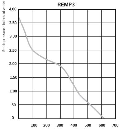
Airflow CFM (Cubic feet/minute)
