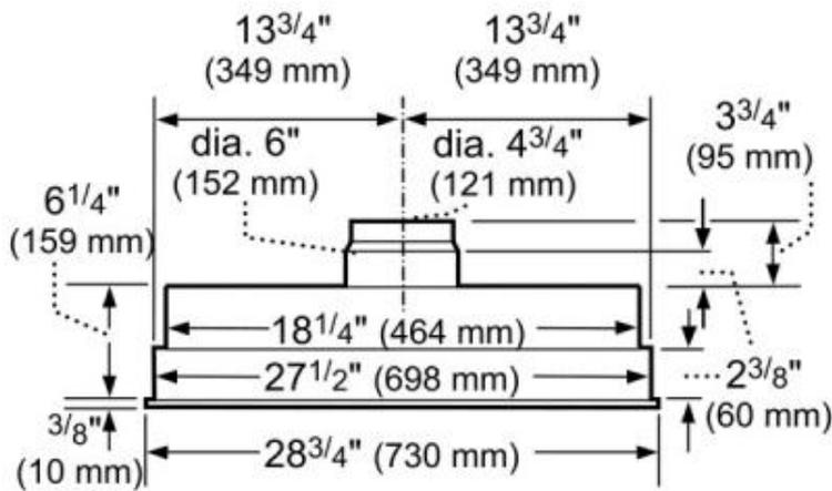
measurements in inches and mm
