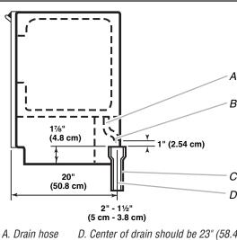
B. 1" (2.54 cm) air gap C. PVC drain reducer
