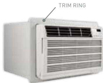
IMPORTANT: 1" gap on sides and 1/2" gap at top, which allows installation into varying sleeve sizes, can be covered by two-piece trim ring that fits over the chassis front. Trim ring comes standard with chassis.
