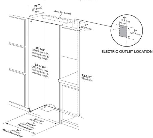
\*Custom panel models fit flush in 25"-deep (63.5 cm) cabinet openings. They can be installed in standard 24"-deep openings. The door faces and top grille will protrude 3/4" (1.9 cm) into the room.
