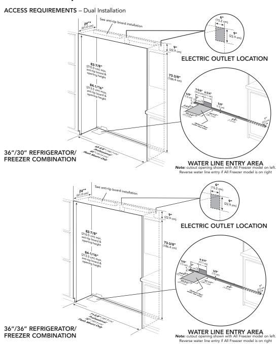
\*Custom panel models fit flush in 25"-deep (63.5 cm) cabinet openings. They can be installed in standard 24"-deep openings. The door faces and top grille will protrude 3/4" (1.9 cm) into the room.
