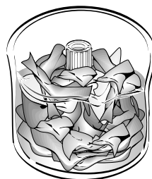
Wrong Water Level for Size of Load
