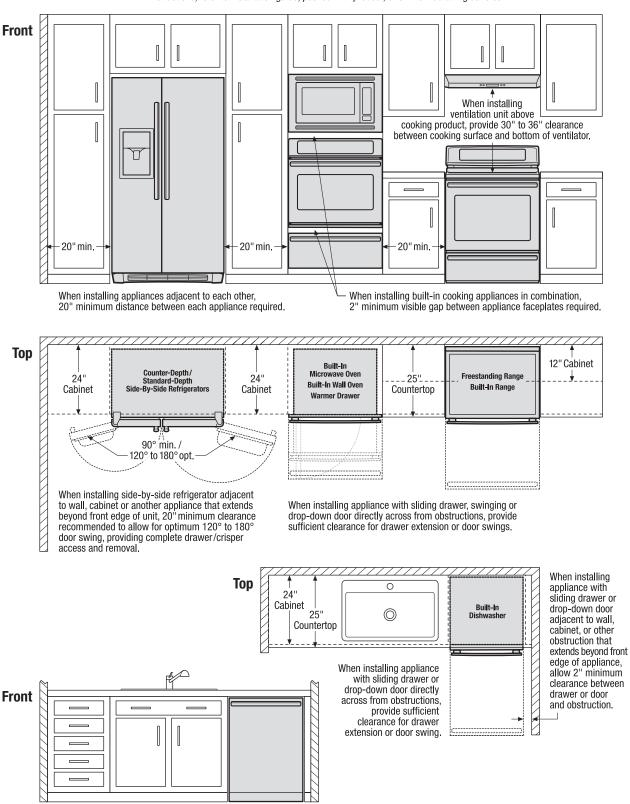
Use these dimensions and clearance instructions for planning purposes only. For detailed installation instructions, refer to installation guide, packed with product, or on the web at frigidaire.com.
