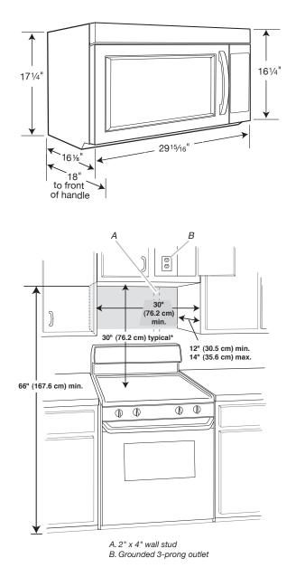
NOTE: The grounded 3 prong outlet must be inside the upper cabinet. \*30" (76.2 cm) is typical for 66" (167.6 cm) installation height. Exact dimension may vary depending on type of range/cooktop below.
