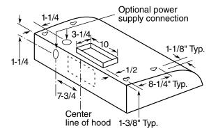
Exhaust outlet connects to 3-1/4" x 10" rectangular duct. Vent top or rear. Includes rectangular damper.
