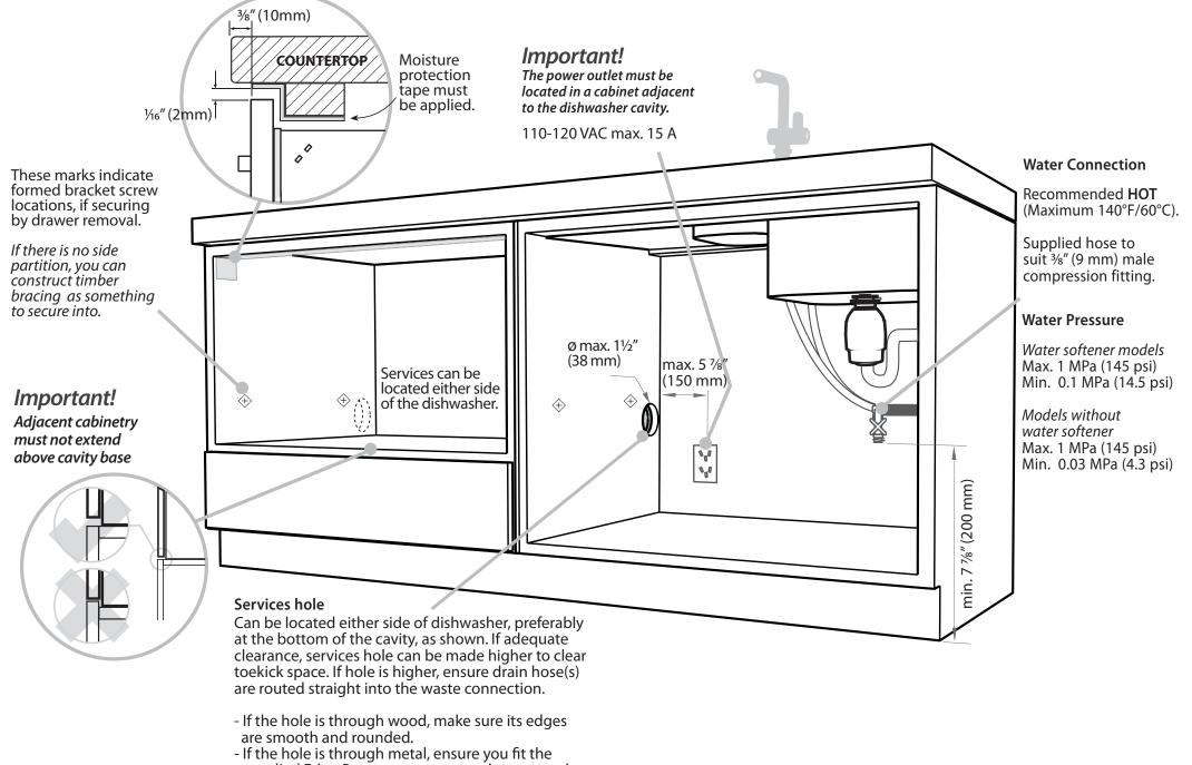
supplied Edge Protector to prevent damage to the power cord.
