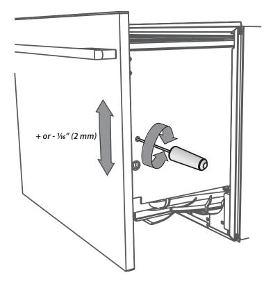
Insert an appropriately sized Philips screwdriver into the hole above the door pin and rotate the panel up or down to align the gaps in your cabinetry.
