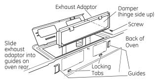
Push down securely until it is in the lower locking tabs. Take care to assure the damper hinge is installed so that it is at the top and that the damper swings freely.
