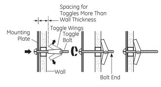
Place the mounting plate against the wall and insert the toggle wings into the holes in the wall to mount the plate.
