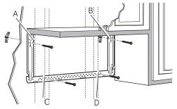
Attach the plate to the wall using toggle bolts. At least one wood screw must be used to attach the plate to a wall stud. Recommended locations on the mounting plate are indicated by A, B, C and D.
