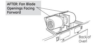
**NOTE:** Make sure wires remain routed in the grooves of the motor frame.
