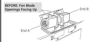
Roll the blower unit 90° so that fan blade openings are facing out the back of the oven.
