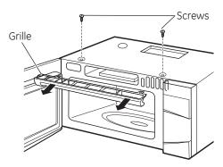
Insert the filter into the oven as shown until it fits squarely into place. It will rest at an angle behind the front lower tabs. When properly installed, the wire mesh of the filter should be visible from the front.
