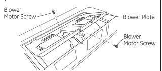
2 Carefully pull out the blower unit. The wires will extend far enough to allow you to adjust the blower unit.
