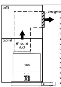
Some ductwork must be installed to exhaust the rangehood back into the kitchen, either at the top of the cabinet or at the face of the soffit. A plastic vent grate supplied with the rangehood can be used to cover the duct opening. This duct work must not terminate into a dead air space.
