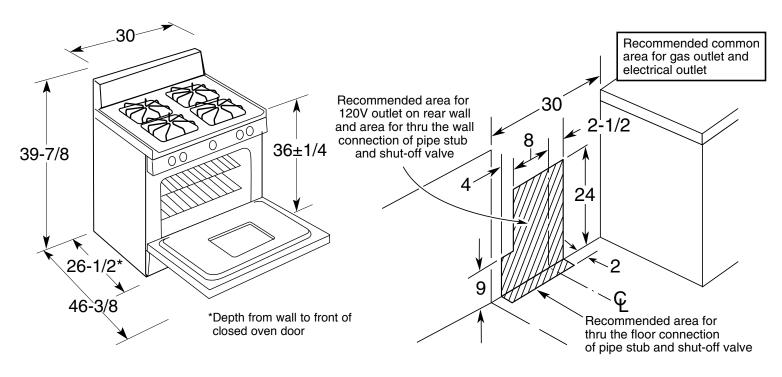
**Installation Information:** Before installing, consult installation instructions packed with product for current dimensional data.
