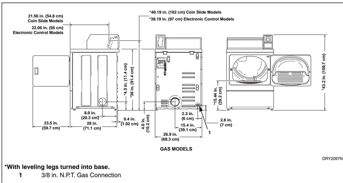
**NOTE:** Side, rear and bottom exhaust openings are 4 inch (10.2 cm) ducting. Gas models cannot be vented out left side of cabinet because of burner housing.
