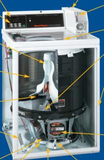
Pump Clips expedite belt replacement. StrongBox Security<sup>TM</sup> features superior meter case to top attachment and top-to-cabinet attachment with greater impact resistance to deter vandalism.
