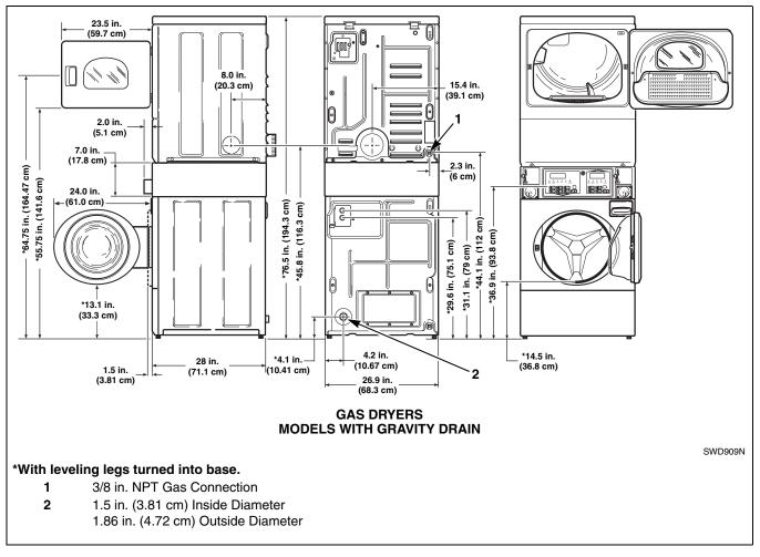
NOTE: Side and rear exhaust openings are 4 inch (10.2 cm) ducting. Gas models cannot be vented out left side of cabinet because of burner housing.
