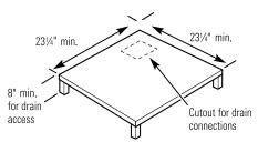
The ZVAC requires a field supplied installation platform. The installation platform must be a minimum of 23 1/4" square, with legs to raise the platform a minimum of 8" (12"
