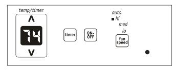
Note: Tap or hold either up (  $\bigwedge$  ) or down (  $\bigvee$  ) button until the desired temperature is seen on the display. This temperature will be automatically maintained anywhere between 60 °F (16 °C) and 90 °F (32 °C) . If you want the display to read the actual room temperature. See "To Operate on Fan Only" section on Page 6.
