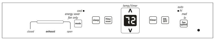
This Exhaust Control allows the air conditioner to either recirculate inside air (CLOSED) or exhaust air to the outside (OPEN). The CLOSED position is used when maximum cooling is desired. It may also be used for air recirculation without cooling when the air conditioner is set in any FAN position.
