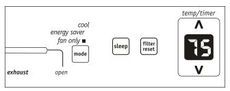
Note: Use this function only when cooling is not desired, such as for room air circulation or to exhaust stale air on some models. (Remember to open the vent during this function, but keep it closed during cooling for maximum cooling efficiency.) You can choose any fan speed you prefer. (Except "Auto Fan").
