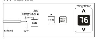
Note: In this mode the selected temperature will increase by 2 °F 30 minutes after the mode is selected. The temperature will then increase by another 2 °F after an additional 30 minutes. This new temperature will be maintained for 7 hours before it returns to the originally selected temperature. This ends the "Sleep" mode and the unit will continue to operate as originally programmed. The "Sleep" mode program can be cancelled at any time during operation by again pressing the "Sleep" button.
