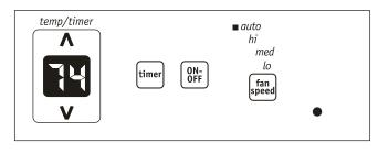
Note: Fan starts at High Speed and adjusts to a slower speeds the room temperature dictates. For example, if the room doesn't get too warm, it will stay at the slowest speed. If the room temperature rises quickly, such as a door being opened, it will automatically go to the highest speed. The fan speeds will re-adjust back to the slowest speed as the room returns to the original set temperature. Press either the fan slower or fan faster button to adjust the fan speed manually.
