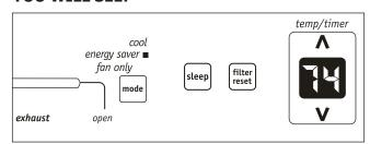
Note: In this mode, the fan will continue to run for 1 minute after the compressor shuts off. The fan then cycles on for 20 seconds at 10 minute intervals until the room temperature is above the set temperature, at which time the compressor turns back on.
