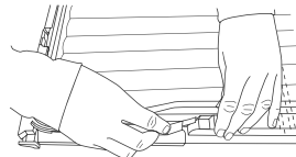
Fig.27 Fit lid under side retainers
