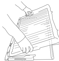
Fig.25 Removing lid from rear clips and side retainers
