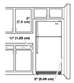
To ensure proper ventilation for your refrigerator, allow for a  $\frac{1}{2}$ " (1.25 cm) space on each side and 3" (7.5 cm) at the top. Allow at least 1" (2.54 cm) between back of cabinet and the wall. If your refrigerator has an ice maker, make sure you leave some extra space at the back for the water line connections.
