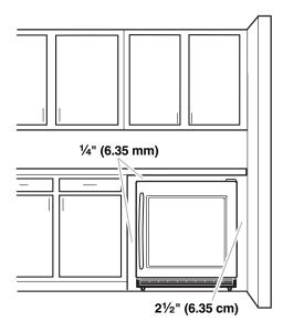
To ensure proper ventilation for your beverage center, allow for a  $\frac{1}{2}$ " (6.35 mm) space on each side and at the top. When installing your beverage center next to a fixed wall, leave  $2\frac{1}{2}$ " (6.35 cm) minimum clearance on each side to allow for the door to swing open.
