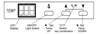
The Light Switch allows you to turn on the interior light with a push of the button. The light will stay on until you push the button again, so be sure to shut it off when not needed, to save energy and avoid raising the cabinet temperature unnecessarily.
