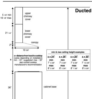
For ducted installations, the chimneys can be adjusted for ceilings between 7' 4 3/8" and 8' 9 3/8" depending on the distance between the bottom of the hood and the cooktop (distance x in Ducted diagram).
