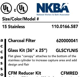
Reduces CFM to under 300 cfm for makeup air environments
