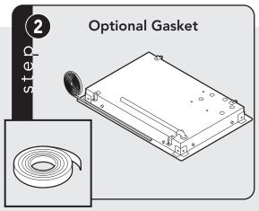
Peel away the plastic covering and place the gasket material all the way around the burner flange.
