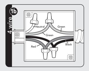
Connect the red, black, and green leads from the unit conduit to the corresponding leads in the junction box.
