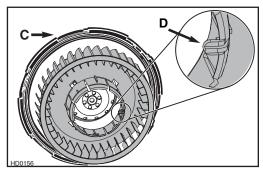
NOTE: Do not try to remove the black part (**C**) attached to the bottompanel. When reinstalling the blower wheel, make sure the small tab (**D**) will fit into one hole of the motor.
