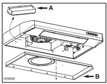
Punch out the electrical and discharge knock-outs for the chosen opening (vertical on top or horizontal at the back of the hood). Refer to figure below.
