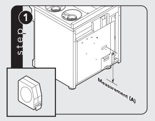
Measure from floor to bottom of the anit-tip opening located on the back of range. This will be measurement (A).
