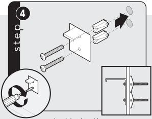
Attach bracket with mounting hardware provided.
