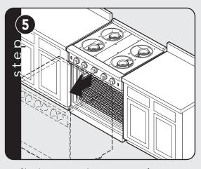
If leveling is required, move unit out of opening.
