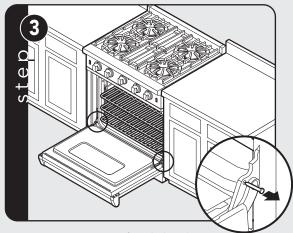
Remove pins from hole in hinges.
