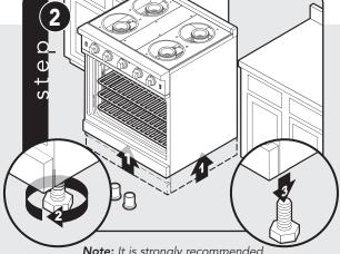
Note: It is strongly recommended that a pallet or lift jack be used rather than tilting.
