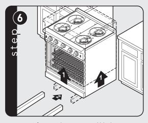
Lift unit and prop on wood blocks.
