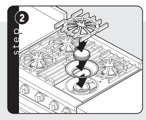
Burner caps and burner bowls are packed in styrofoam top pack with the grates. Place burner bowl in grate support and burner cap on top of burner. Place burner grate over burner cap and on top of grate support.
