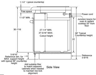
**Note:** 36" ribbon cooktops are approved for use over GE 30" single wall ovens only. 30" ribbon cooktops are approved for use over GE 30" and GE 27" single wall ovens. Refer to cooktop and wall oven installation information packed with products for current dimensional data.
