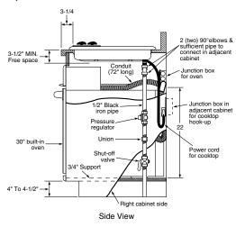
This installation is to achieve minimum gap between bottom of countertop and control panel.
