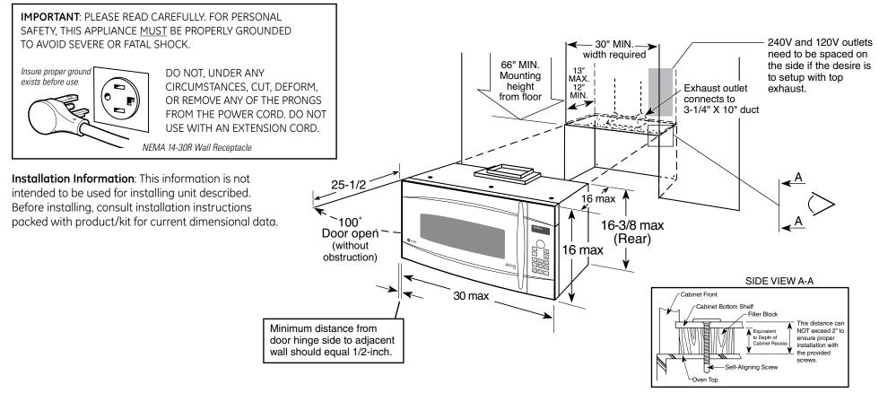
Note: Outside venting is optional. Vent (duct) can be horizontal or vertical.
