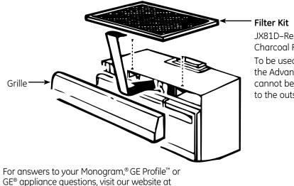
JX81D-Recirculating Charcoal Filter Kit To be used when the Advantium oven cannot be vented to the outside.
