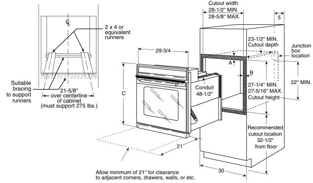
A=Allow 1" overlap of oven over top and bottom edges of cutout. B=Allow 11/16"-3/4" for overlap of oven over side edges of cutout. C=28-1/4" without trim and 28-3/4" with trim.
