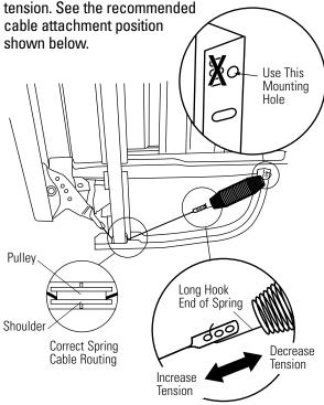
Recommended Position of Spring Hook to Cable Shown
