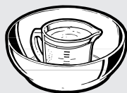
How to test for a microwave-safe dish.
