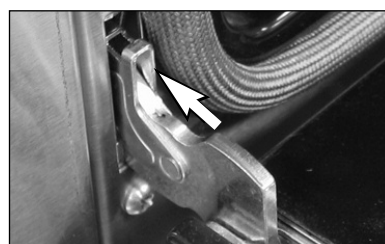
Fig. 25 Hinge retainer clip in locked position
