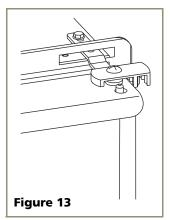
engages the closer in the assembly, then tighten screws on travel pin assembly securely. See **Figure 13**.
