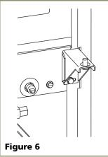
Remove bottom hinge from cabinet (two screws). See
