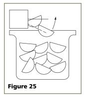
arm into an upright and locked position (see **Figure 25**). While the bin arm is locked, the unit will maintain temperature for ice storage.
