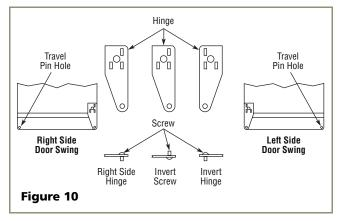
8. Remove pivot screw from top hinge, invert screw and reinstall pivot screw in top hinge. See **Figure 10**.
