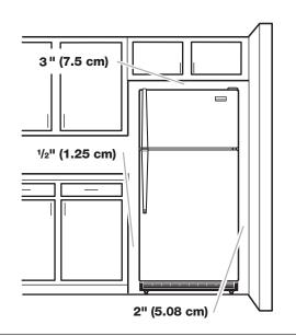
To ensure proper ventilation for your refrigerator, allow for a  $\frac{1}{2}$ " (1.25 cm) space on each side. Allow 3" (7.5 cm) of space between overhead cabinets and refrigerator top. Allow at least 1" (25.40 mm) between back of cabinet and the wall. If your refrigerator has an ice maker, make sure you leave some extra space at the back for the water line connections.
