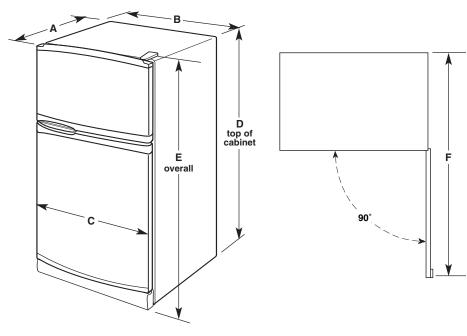
Dimensions "D" and "E" include rollers extended ¾" (1.9 cm)
