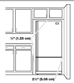
To ensure proper ventilation for your refrigerator, allow for a 1/2" (1.25 cm) space on each side and at the top. Allow at least 1" (2.54 cm) between back of cabinet and the wall. If your refrigerator has an ice maker, make sure you leave some extra space at the back for the water line connections.
