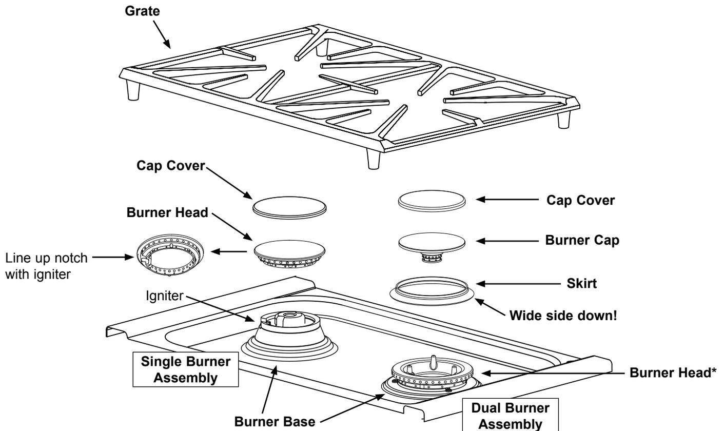
\* The burner head on the dual burner assembly is permanently attached to the burner base. It cannot be removed by the customer.
