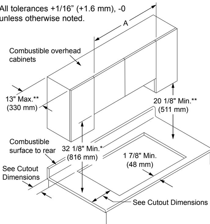
\* If installing with an overhead vent hood, also check the hood specifications for minimum required clearances.
