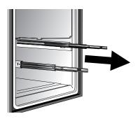
**Note:** All four drawer bracket supports must be in the proper slots for the drawer to function properly.
