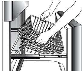
3. On each white drawer bracket is a basket cradle with two snap attachments. To release each cradle, unlatch the snaps by pushing them inward, away from the side bracket. Lift the cradles off of the rails.
