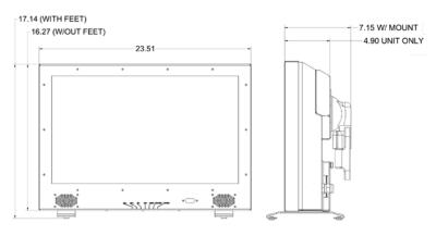
23.51 in. W x 16.27 in. H x 4.90 in. D Height dimension with table stand is 17.14 in. TV with optional wall mount measures 7.60 in. when folded flush against the wall.
