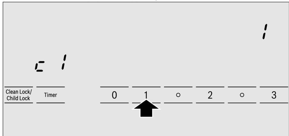
5. Press the **Timer** symbol again for more than 4 seconds, until you hear a sound signal. The settings have been correctly stored.
