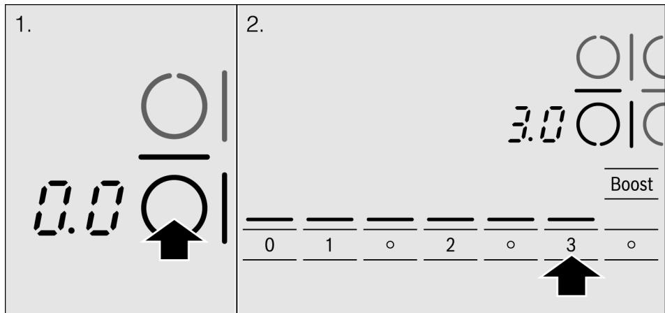
3. To change the heat setting: Select the element and then press the symbol for the required heat setting. To select an intermediate level, press the o symbol which is located between the heat setting symbols.
