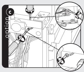
Loosen ground wire and wires on terminal block.
