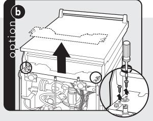
Remove bottom pan and front plate.
