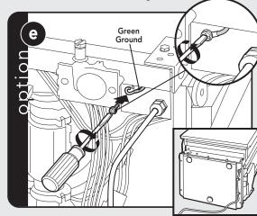
Connect ground wire. **NOTE:** Reinstall front plate and bottom pan.
