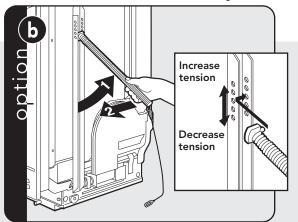
Set counter balance spring connector in appropriate
