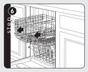
To check level, front to back, pull the top rack half-way out of unit. The rack should remain stationary and not move in or out.
