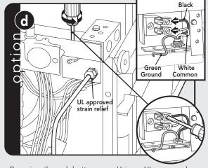
Run wires through bottom pan. Using a UL approved strain relief, connect wires to terminal block.
