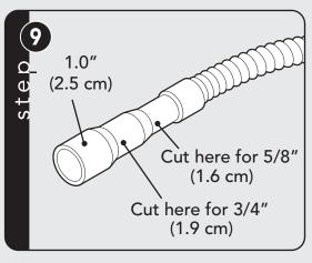
Identify discharge connection size; cut line to correct size and connect. Clamp if necessary.
