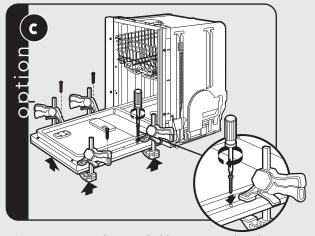
Use non-marring clamps to hold custom panel in place. Secure with #8 1-3/4"(4.5 cm) long, stainless steel flat head screws.
