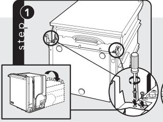
Carefully lay dishwasher on its back and attach the kick plate brackets. Screws for the brackets will already be in the base. **NOTE:** Be careful not to pinch hoses or power cord beneath dishwasher.
