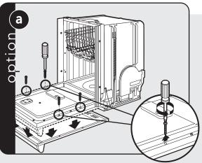
To remove face panel of dishwasher remove only the 4 Phillips screws - do not remove any other fasteners.
